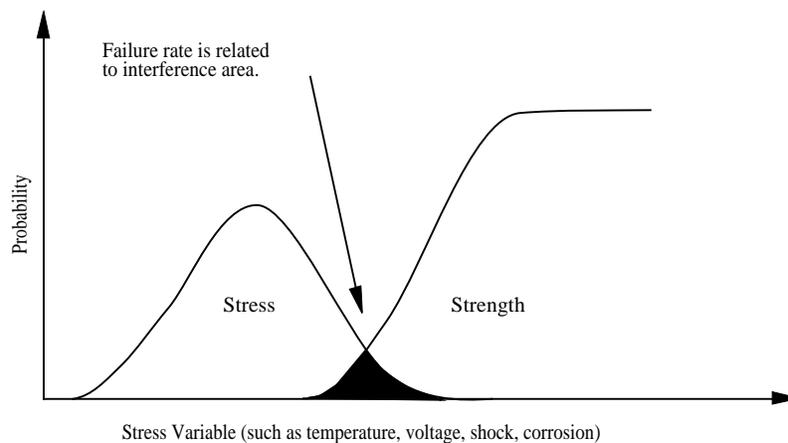
Figure 1 Stress/strength interference
