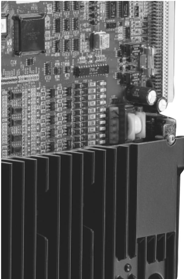
**Figure 4** Module cutaway showing protection against heat
