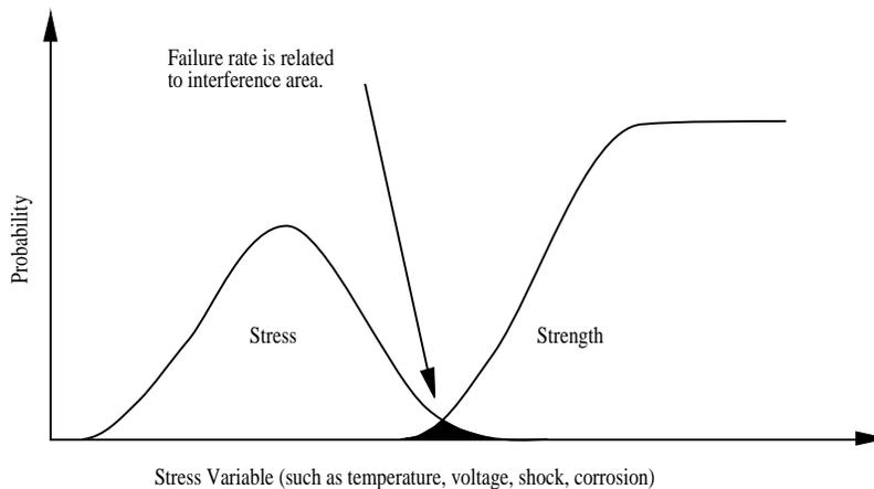
**Figure 3 Higher strength, lower failure rate**
