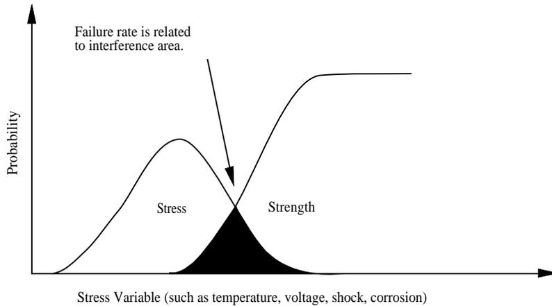
**Figure 2 Lower strength, higher failure rate**
